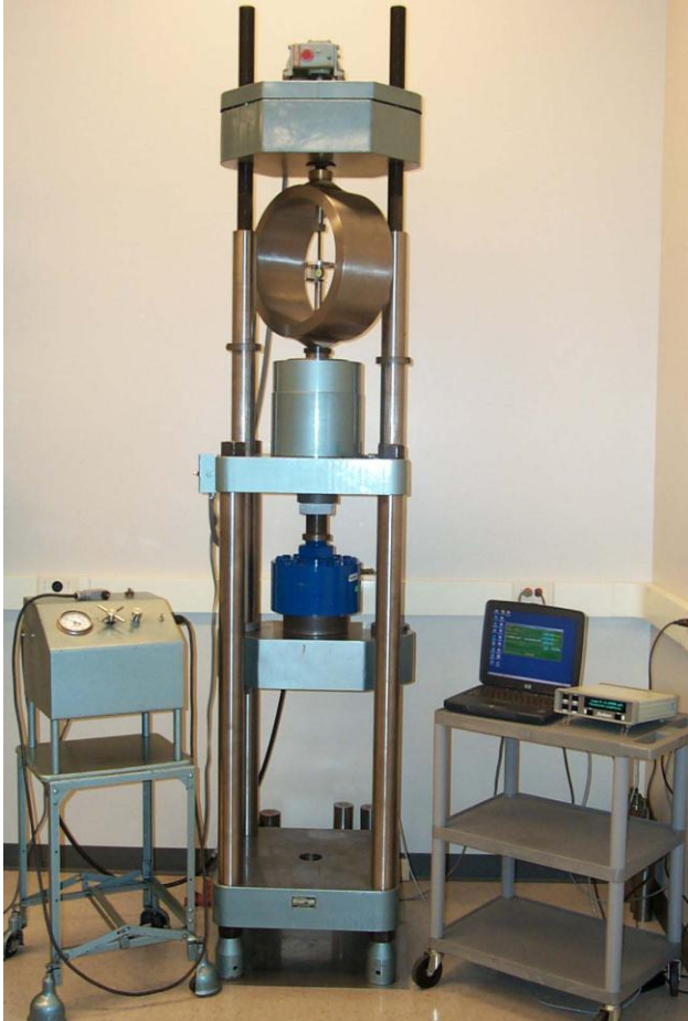
(pictured above 300,000 LBF Universal Calibrating Machine setup with 200,000 LBF Series 1000 Proving Ring, Hydraulic Power Control, Morehouse Calibration Meter and Morehouse software which converts mV/V values using coefficients generated from a curve fit equation to allow true direct reading in LBF, N or KG.)
